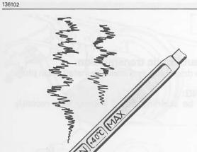
**Check condition of Automatic Transmission Fluid.** Fluid must not carry impurities, discoloration or smell.
