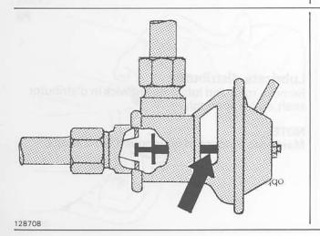
2. Warm engine, coolant temperature above + 60° C. EGR valve should open at rpms above idle speed with warm engine.
