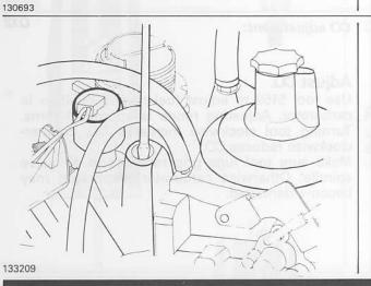
Adjust idle speed. Engine at normal operating temperature. During and after CO adjustment, idle speed should be: 900  $\pm$  50 rpm.
