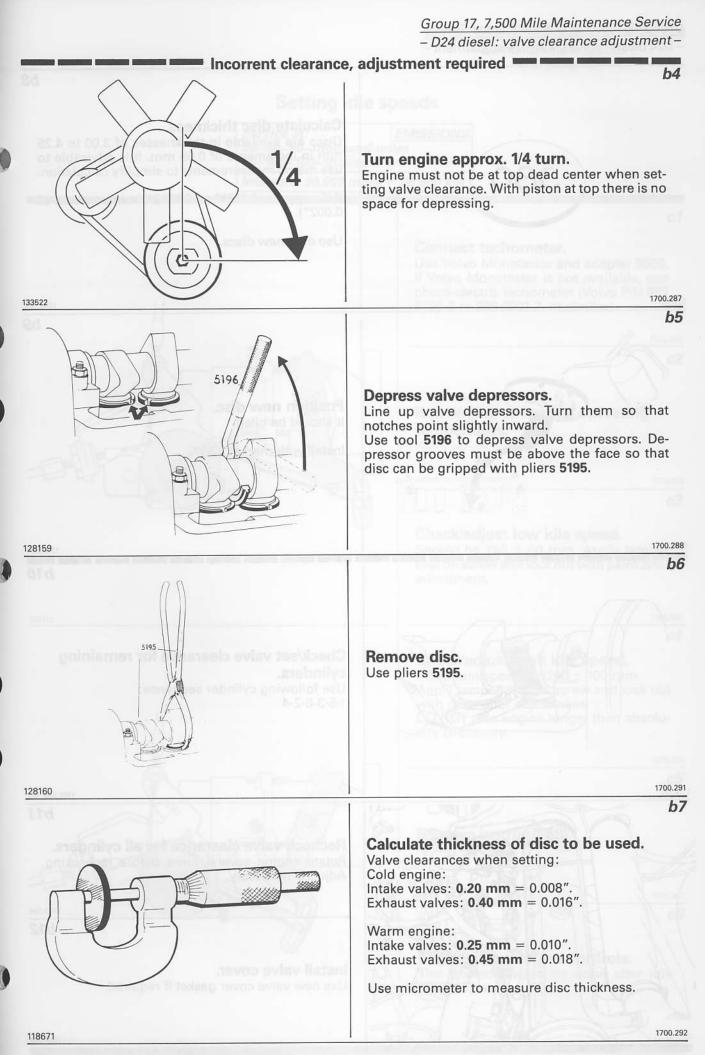
Group 17, 7,500 Mile Maintenance Service – D24 diesel: valve clearance adjustment –
