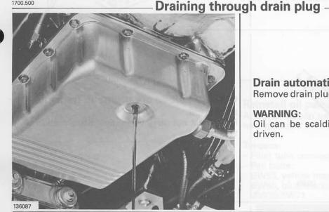
Drain automatic transmission. Remove drain plug and drain. Reinstall drain plug.
